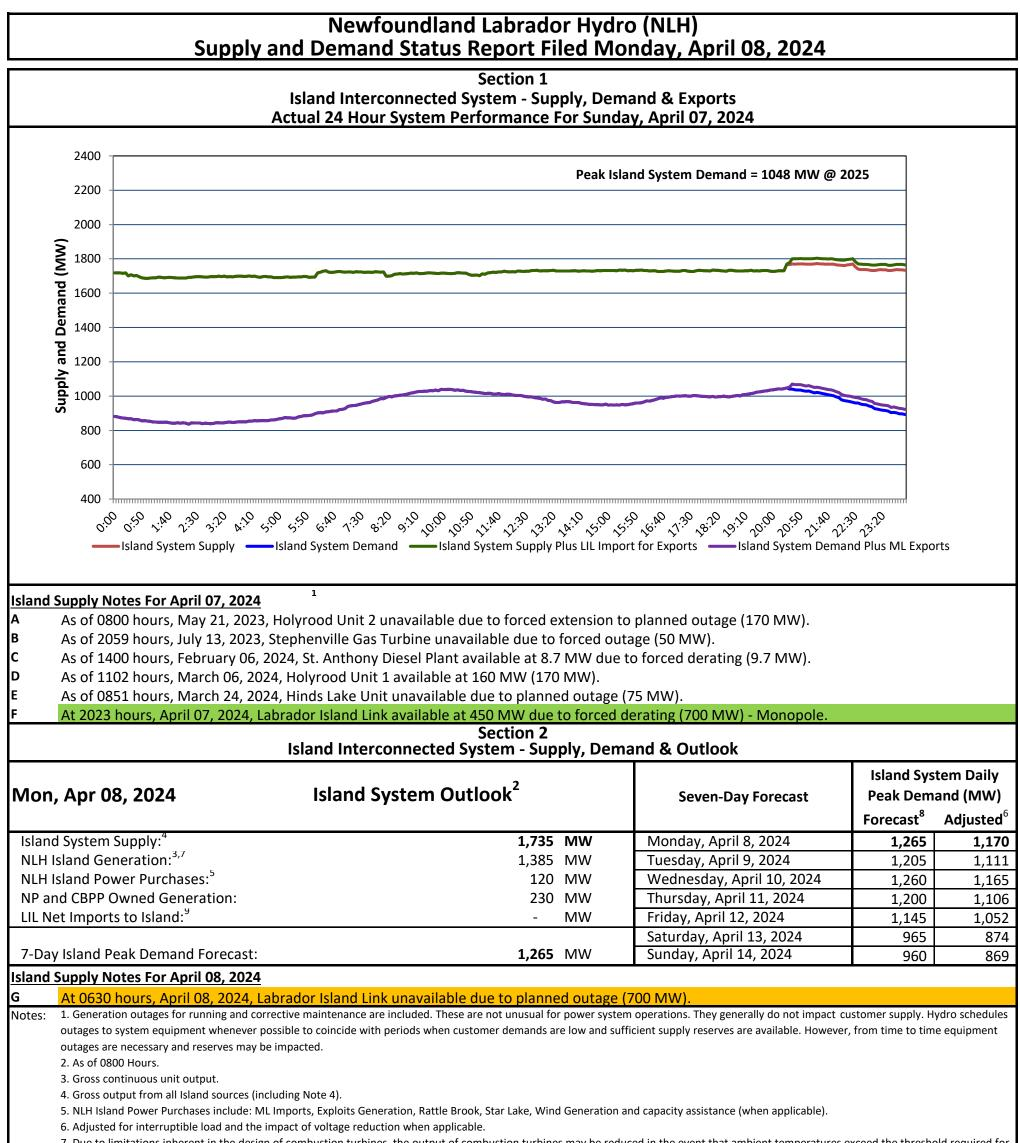
7. Due to limitations inherent in the design of combustion turbines, the output of combustion turbines may be reduced in the event that ambient temperatures exceed the threshold required for full rated output. This threshold is dependent on the design of each turbine.
